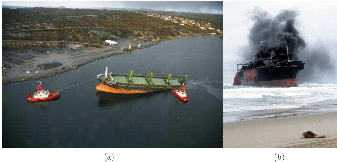
Figure 1.1: (a) shows the bow and cargo section of “ MS Server ” which broke in two outside Fedje, Norway, after grounding. Fig (b) shows a photo of the “ New Carissa ”, which run aground at the US west coast.
